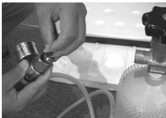
Illustration A Black Rubber Washer Installed in Wing Nut
